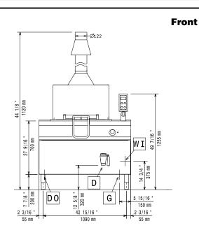
D = Drain WI = Water inlet EI = Electrical inlet (power)
